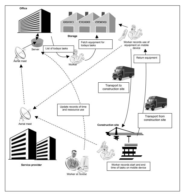
Figure 4 Physical model of the situation after introduction of the mobile resource management system at company 3.
