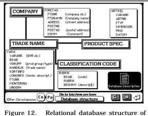
Figure 12. Relational database structure of the facts base in the AMVI system. A detailed record description is found in table 1.
