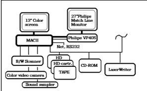
Figure 3. Hardware components in the KBS-MEDIA environment. MacII computers from Apple Computer. Scanning by B/W scanner, sound sampler and digitizing from Super-VHS camera. 45 Mbyte hard disk cartridge are extensively used for storage. The Videodisk player may also display its output on the computer screen making the image and video films touch sensitive.
