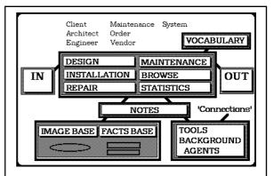
Figure 5. Logical layout of a demonstrator of the material vendor information system. Three levels are distinguished: The context level with different views (design, installation etc.) to the system, the facts bases and tools/background agents and the intermediate notebook or short term memory.
