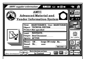
Figure 6. The in-context describing the user, view to the system, type of vendor target product (if any) as well as settings about access levels, output specifications and system performance. The screen display corresponds to the "IN" box of figure 5.
