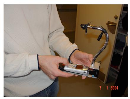
Figure 4 Ericsson T68i Mobile phone mounted on video stand for capture of mobile phone keyboard and screen. The video camera is wirelessly connected to video recording device.
